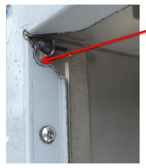
Open the front door and install the surround with rounded cutouts at the top as shown.
